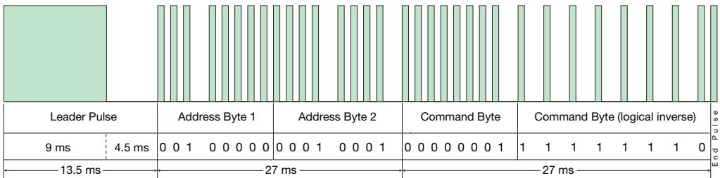
Figure 6-1. NEC Protocol Message Format
